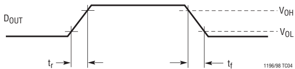
Voltage Waveform for D_{OUT} Rise and Fall Times, t_r , t_f
